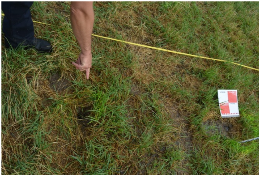
Figure 6 Identification of exit point
