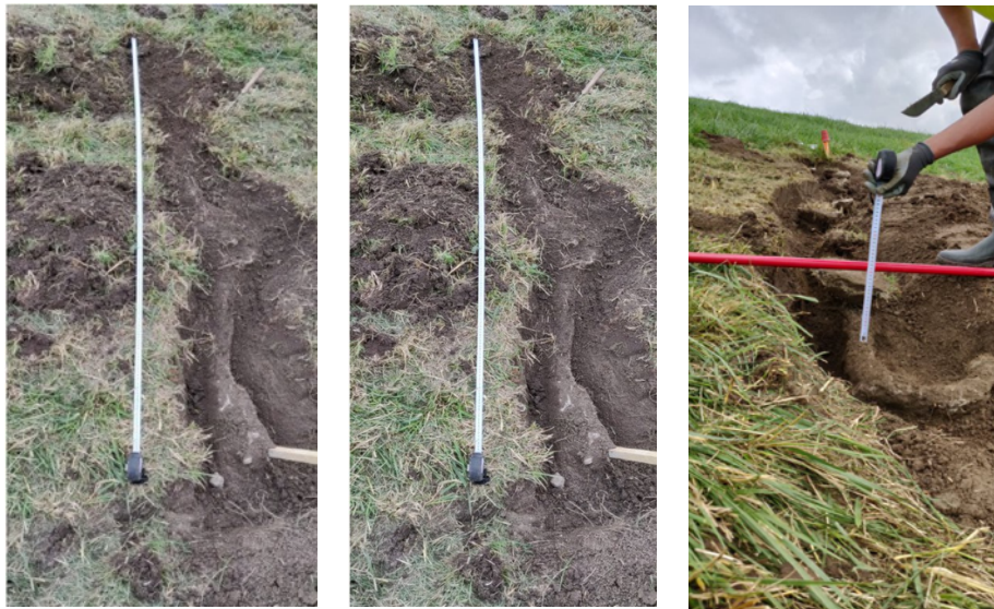
Figure 15 a) Length measurements of focus area b) depth measurements of burrows. c) depth measurements of cracks
