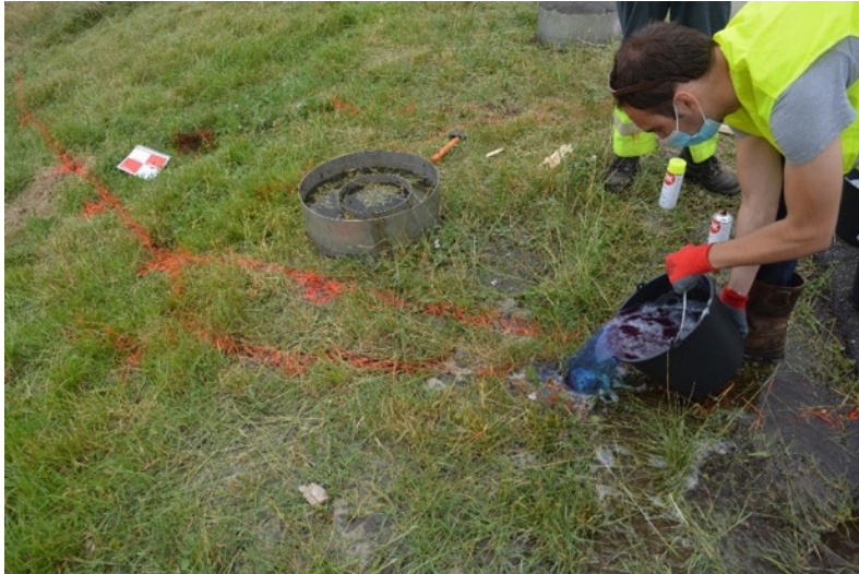
Figure 12 Application of colourant to find preferential flow paths
