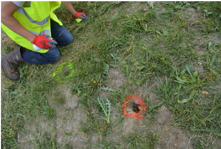
Figure 9 Marking burrows and discontinuities that are suspected from human interventions (Yellow) or from animal activities (Orange)
