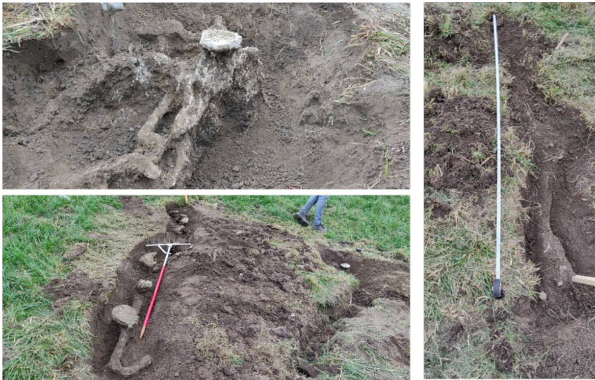
Figure 17 Upper left: Hardened concrete was at 50 to 55 cm depth. Because of the combination of cracks and mice burrows the exact depth cannot simply be attributed to either one of them (Focus location The Netherlands 3). Lower left Interrupted concrete structure indicating the recovering of a crack (Focus location The Netherlands 2). Right: Mole burrow longer than 4m ((Focus location The Netherlands 1).
